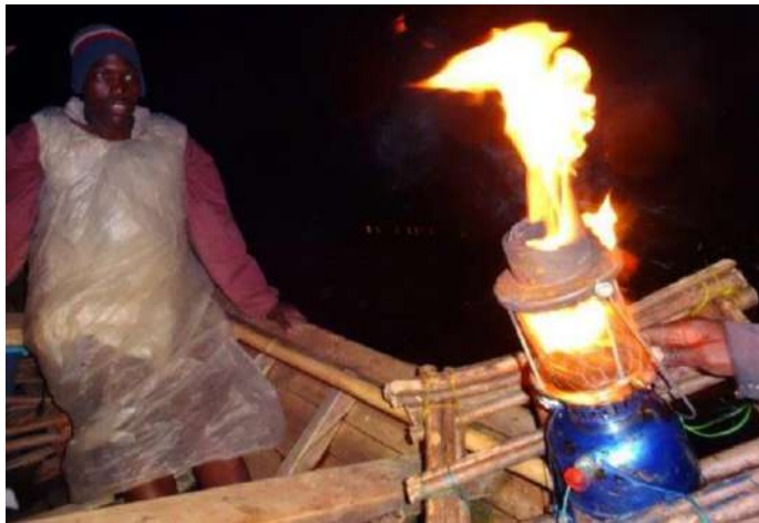
Photo 4: Accident, exploded pressurized kerosene lantern ©TAREA
