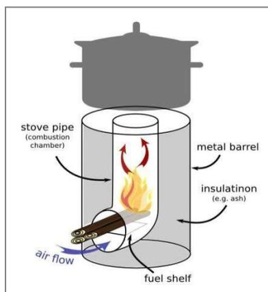
Figure 3: Schematic illustration of the rocket stove cooking system (Source: <http://en.wikipedia.org>)
