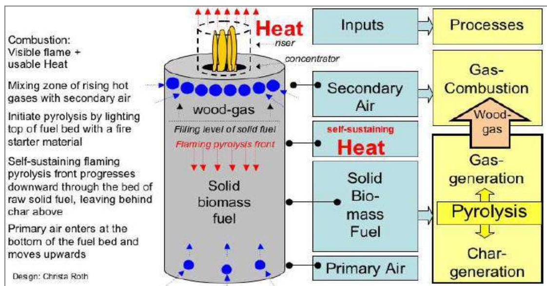
Figure 2: Principle of Top-Lit Updraft (TLUD) Gasifier Stove<sup>9</sup>
