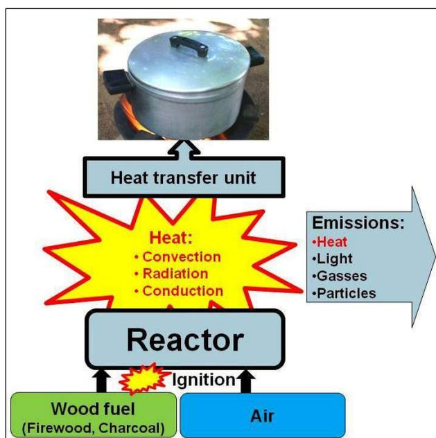
Figure1: Schematic illustration of stove cooking system (Source: <https://energypedia.info/>)
