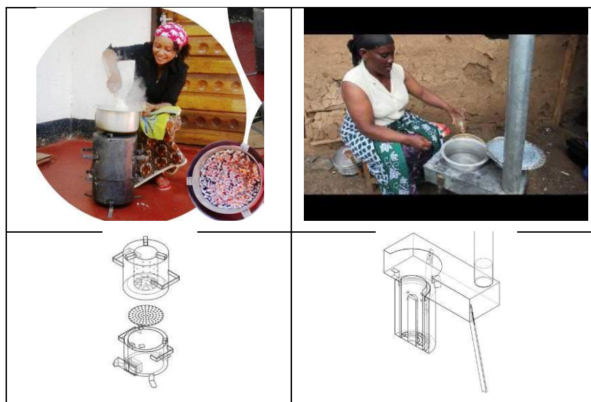
Figure 5.3 Jiko Bomba (left) and Jiko Safi (right) gasifier stoves
