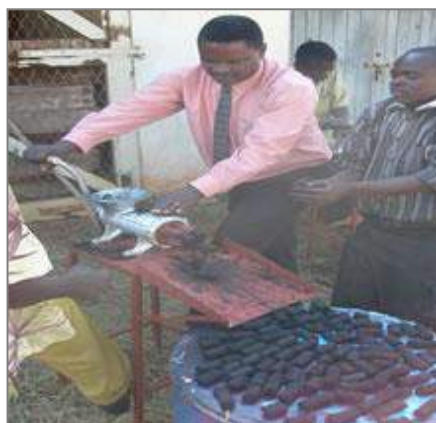
Making of charcoal briquettes at Nishati Poa (Arusha)
