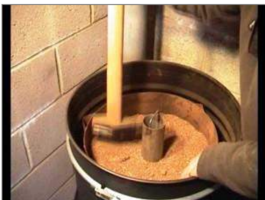
Compaction of sawdust before igniting the semi-gasifier stove
