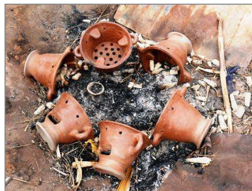
Curing of clay stoves using maize cobs at Mafinga (Iringa region)
