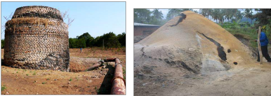
Figure 7.19 Disposal system for coffee husk at Mbozi coffee mill (L) and rice husks open burning behind the mill in rural Morogoro (R)
