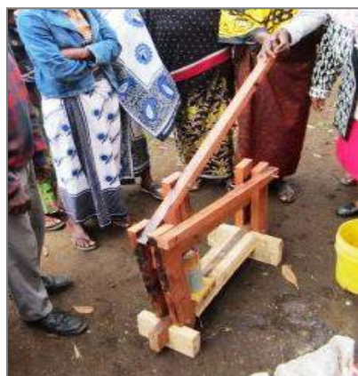
Hand-operated briquetting machine used by Mkombozi Women Group (Lushoto)
