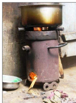
Cooking with semi-gasifier stove
