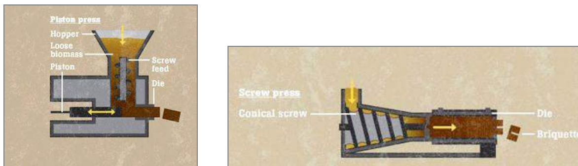
Figure 7.2 Schematics of piston (L) and screw (R) briquetting machines
