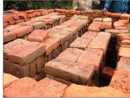
Arrangement of Bricks in Kiln using Rice Husk
