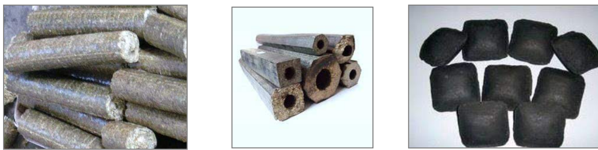
Figure 7.4 Briquettes from piston press (L), screw press (C), and roll press (R)
