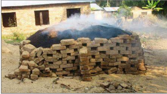
Brick Kiln using Rice Husk
