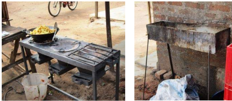
Figure 3.2 Photos of tradition charcoal stoves (R) and ICS (L) used by food vendors
